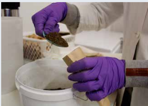
Sampling of copper-contaminated vineyard soils after a 6-month simulation of climate change to determine chemical and microbiological changes in the soil.
