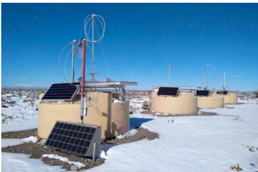
The upgraded surface detector stations of the Pierre Auger observatory with a plastic scintillator on top, providing composition sensitivity of primary particles. An additional antenna will enhance composition sensitivity at large zenith angles.
