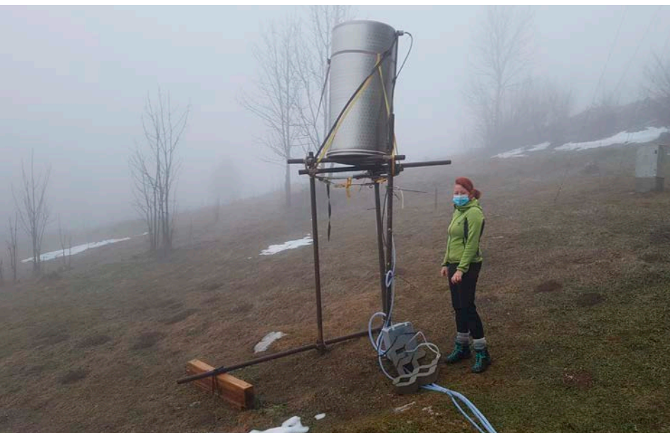
Measurements of aerosols, water droplets and ice crystals in clouds at the Otlica observatory.
