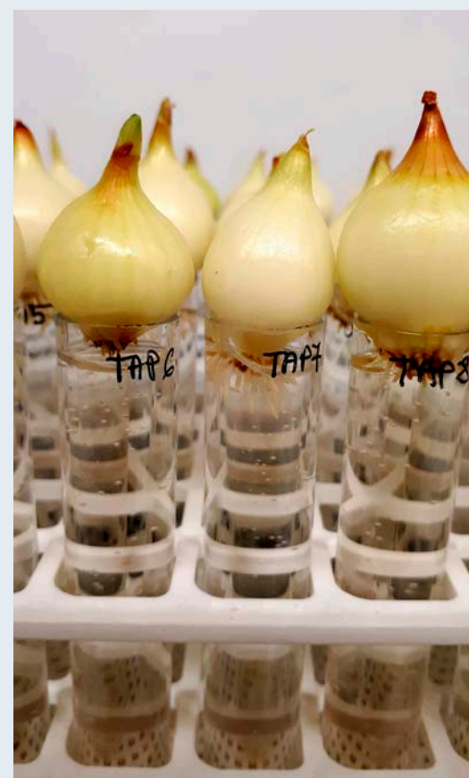
Allium test with waste water, treated by using an electrochemical approach (done in MRL lab).
