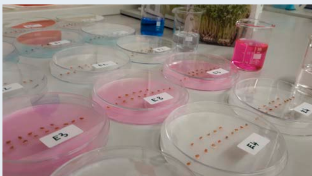
Lepidium sativum germination test with model waste water, treated by using an electrochemical approach (done in MRL lab).
