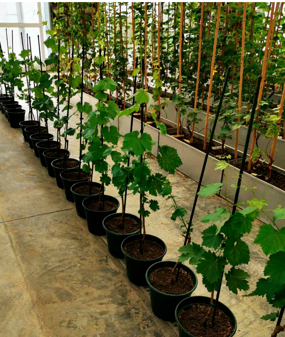
Pot experiment set-up for performing irrigation experiment with treated waste water.
