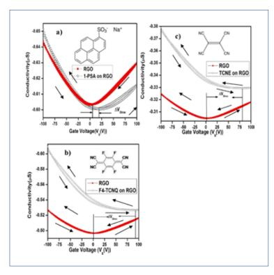
The figure shows the normalized conductivity as a function of gate voltage for a field effect transistor based on graphene oxide (RGO) when a) 1-PS, b) TCNE and c) F4-TCNQ were deposited.
