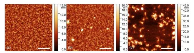
The figure shows surface measurements using the atomic force microscope on samples of a) pure P3HT, b) P3HT with 0.2% graphene nanoparticles and c) P3HT with 3.2% graphene nanoparticles.
