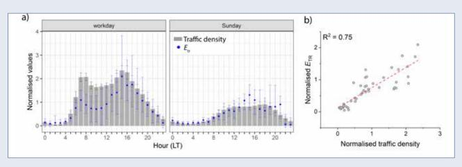
The determined emission rates for traffic E, which is independent of the weather, and agrees well with the traffic counts in Ljubljana (Gregorič et al., 2019).
