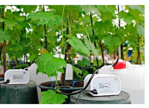
Pot experiment with vine plants irrigated with the tap water, with the treated model waste water, cleaned with electrochemical approach, and with the model waste water.
