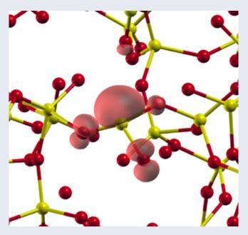
Spin-density (shaded) of the P1like configuration obtained after placing an extra PO, unit nearby a nonbridging oxygen in a P<sub>2</sub>O<sub>5</sub> glass model.
