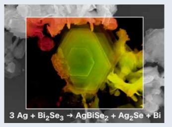
Elemental mapping of Bi<sub>2</sub>Se<sub>3</sub> particles with Ag deposition showing chemical reaction and formation of new phases. Similar reactivity was observed with Ti applied.
