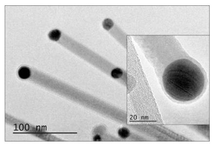
TEM image of Ga-Se nanowires with gold nanoparticles at the tip. In the inset, magnified detail of the tip. A novel strategy is developed to simultaneously fight plastic pollution, cleaning water and producing hydrogen via water splitting. At first, the fluorescent carbon quantum dots (CQDs) were fabricated from polyethylene: popular plastic source and designed to act as a metal nanosensor (Cu@CQDs) for cleaning waste water. Further, the solution of Cu@CQDs was im-
