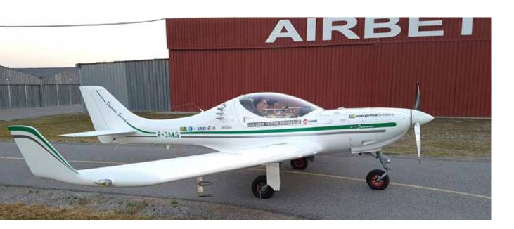
The aircraft with the equipment for measurement of pollutant vertical profiles. We see the fine aerosol inlet under the wing and the coarse aerosol inlets on the fuselage.
