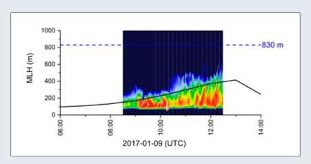
The comparison of lidar- and model-derived (black line) mixing layer height. The model uses measurements of the radon concentrations to derive the height, which agrees well with the lidar measurements (Gregorič et al., 2019).
