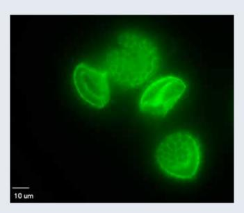
Structure of sporopollenin microcapsules acquired by fluorescence microscope (640x magnification).
