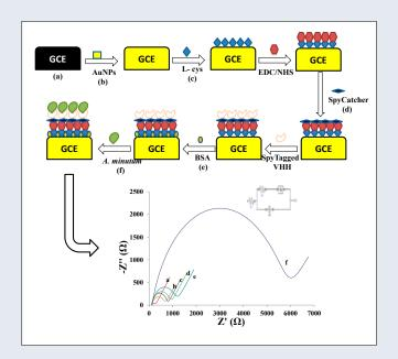
Schematic representation of the biosensor preparation and of the dose-dependent electrochemical impedance response.
