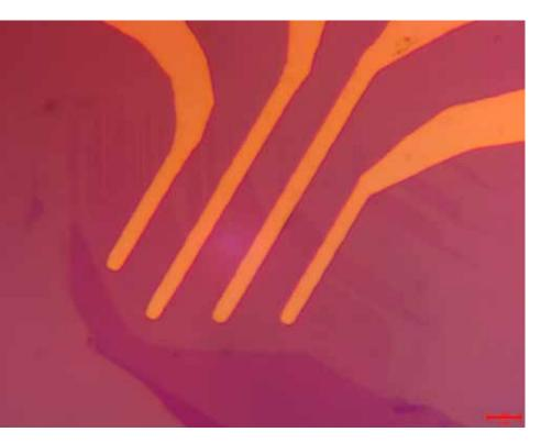
Optical micrograph of metallic contacts on a single-layer graphene flake.
