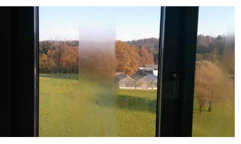
Antifogging thin film on window: less active left, more active right, no coating in the middle.
