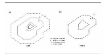
Discretisation scheme of classical method of fundamental solutions (a) and method of regularized sources (b).
