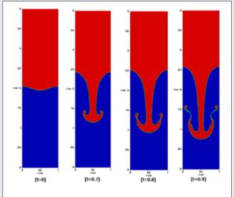
Simulation of instability of two fluids. The fluid with larger density is on the top and the fluid with the lower density os on the botom. The surface tension has been taken into account.
