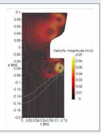
Simulation of flow structures in direct-chill casting of aluminium alloys. Without influence of electromagnetic field (left). With influence of elecromagnetic field (right).
