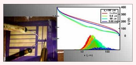
Position dependence of electric potential and density of photogenerated charge carriers in organic semiconductor between coplanar electrodes. Each curve represents the results of Monte Carlo simulation using different time delay from the carriers photogeneration. The background represents a photo of the measurement of the time-dependence of photogenerated current.
