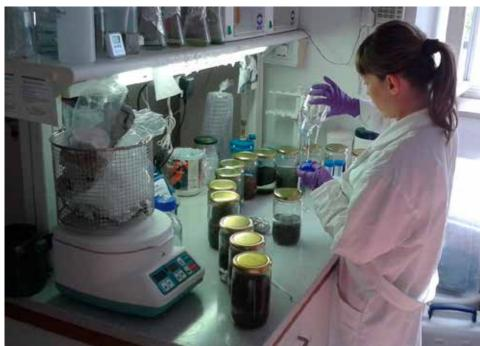
Laboratory work: testing of different materials for adsorptive ability
