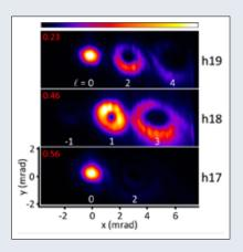
Transverse profiles of the ring-like shaped optical vortices obtained at CITIUS with the two-color wave-mixing scheme. For each harmonic (h) of the driving laser, the OAM content (l) can be controlled by adjusting the intensity of the two driving lasers.
