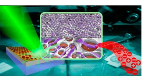
Perylene-carboxiimde (PTCDI-C8) nanowires on top of hexagonal nanostructures, which acts as a very sensitive photodetector for visible light. Since nanoscale dimensions, the photocurrent response is in the range of few nanoseconds.
