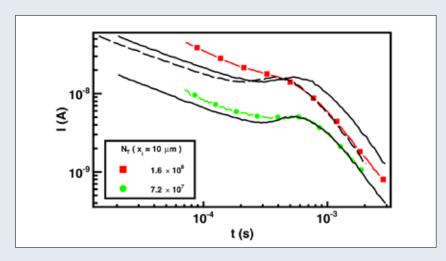
Time-dependence of photoexcited charge carriers current in polythiophene (P3HT) nanowires. Curves exhibit a double cusp. The first cusp occurs at shorter times due to arrival of the carriers drifting through ordered nanowires. In contrast, the second cusp occurs at longer times due to slower transport through disordered polymer regions. At higher bias voltage, the transit times reduce due to higher carriers velocity.
