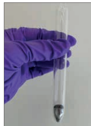
Synthesized high-quality \text{Bi}_{1.2}\text{Mn}_{0.9}\text{Se}_{4.2} single crystal prepared by the Bridgman method.
