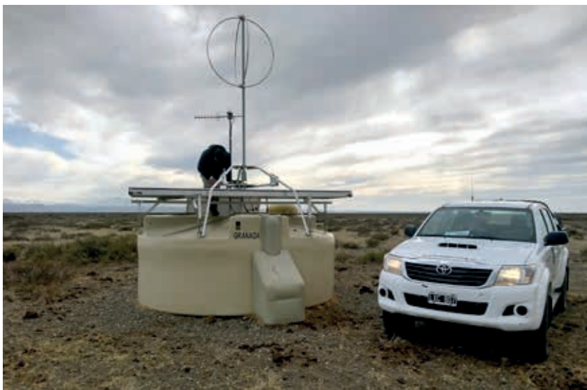
The final upgrade works on Pierre Auger surface detector stations with a plastic scintillator on top, providing composition sensitivity of primary particles, and an additional antenna to enhance composition sensitivity at large zenith angles.
